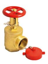
HC-103(DWG.J282) Pressure Reducing Device Angle Valve 175 Lb. Rated Adjustable restriction of residual pressure up to 175 lb. Locking pin device restricts full opening of valve by untrained personnel, pin may be removed by firefighters to allow full opening of valve. FEMALE x MALE
